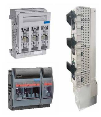
NH stands for "low voltage high rupturing capacity" (from the German: Niederspannungs Hochleistungs Sicherungen). NH fuses have a breaking capacity generally exceeding 100 kA, which covers virtually all the short-circuit currents expected to be encountered in low voltage systems.
