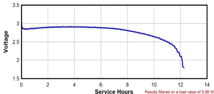
Internet Camera Testing 560mW Pulse Testing to 1.8 Cut-Off
